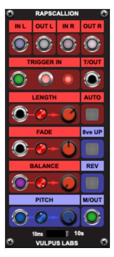
Rapscallion's controls fall into two colour-coded sections. The **red** section controls the behaviour of the audio gate, and the **lilac** section controls the behaviour of the mod signal. Unless you're connecting **Rapscallion** to **Catkins/Stereo**, you're not going to need the lilac section at all.
