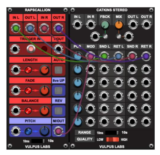
In this configuration, the send/receive loop of the first **Catkins Stereo** delay tap is routed through **Rapscallion**'s audio gate, and **Rapscallion**'s mod output modulates the position of the read head for the delay tap. Note the agreement between the positions of the **RANGE** switches on both modules - this is important for correct pitch-shifting behaviour.
