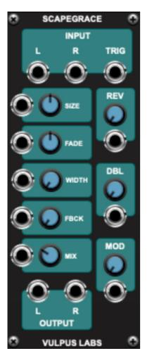
The **L** and **R** jacks in the **INPUT** section of the module are for the left and right input signals. If only the left jack is connected, its input is copied over into the right channel.
